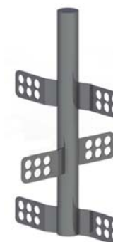
Blades on the central shaft
